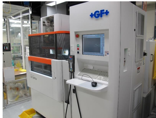
Figure 13. The wire EDM system installed in LAMDA to manufacture specimens from radioactive material.
