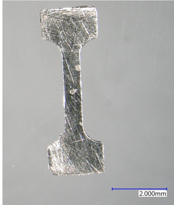
Figure 14. Miniature tensile specimen extracted from the 304D-5-14 friction stir weld metallographic specimen.
